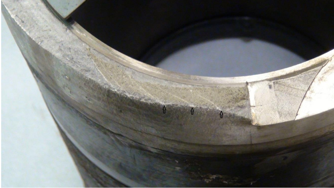
Figure 3.1. Test specimen with arrows annotating the unload marks.
