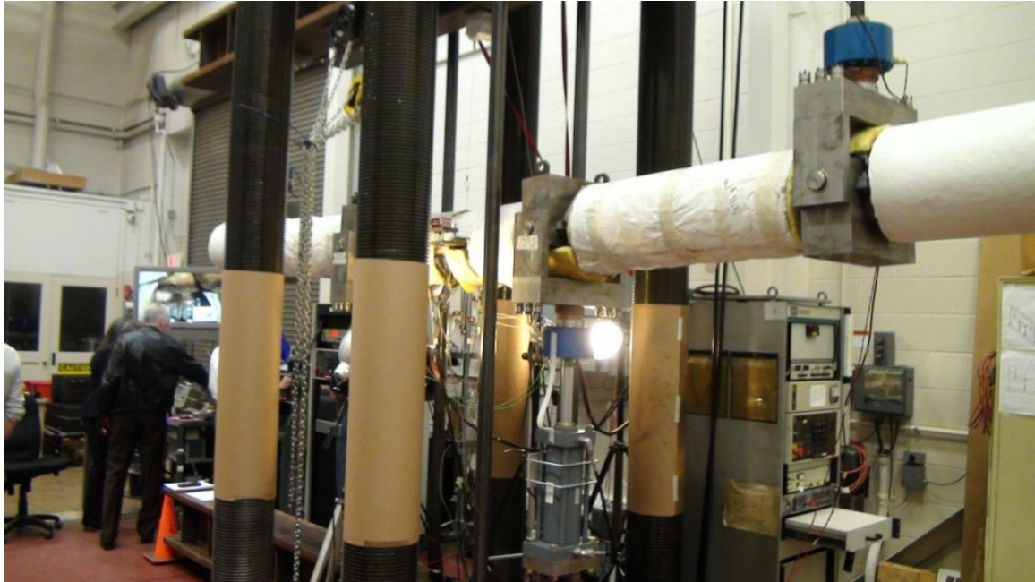
Figure 3.2. 500 kip MTS servo-hydraulically controlled test frame in Battelle's Fatigue and Structures Laboratory.
